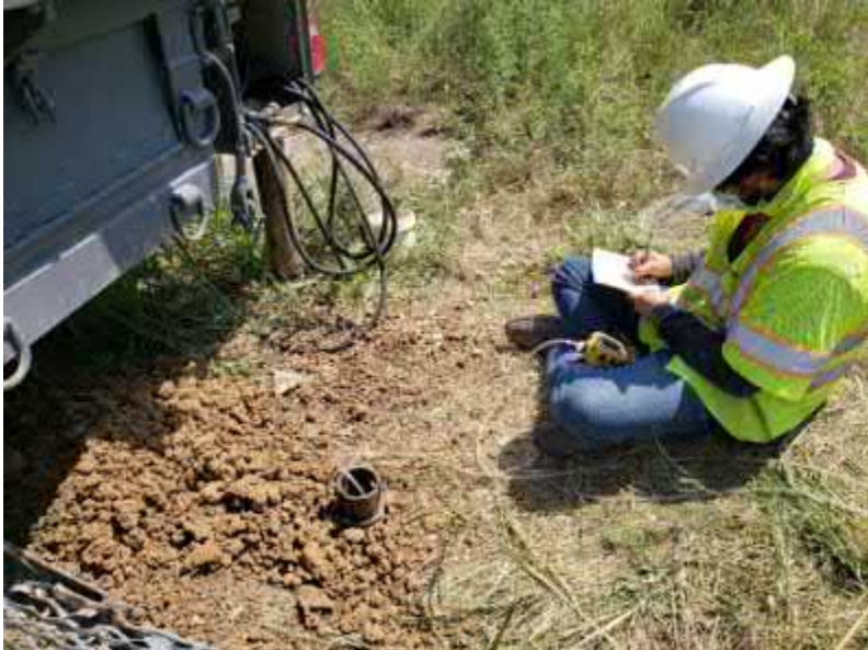
Photo #5 View of technician collecting down-hole methane readings at soil boring MM-2.
