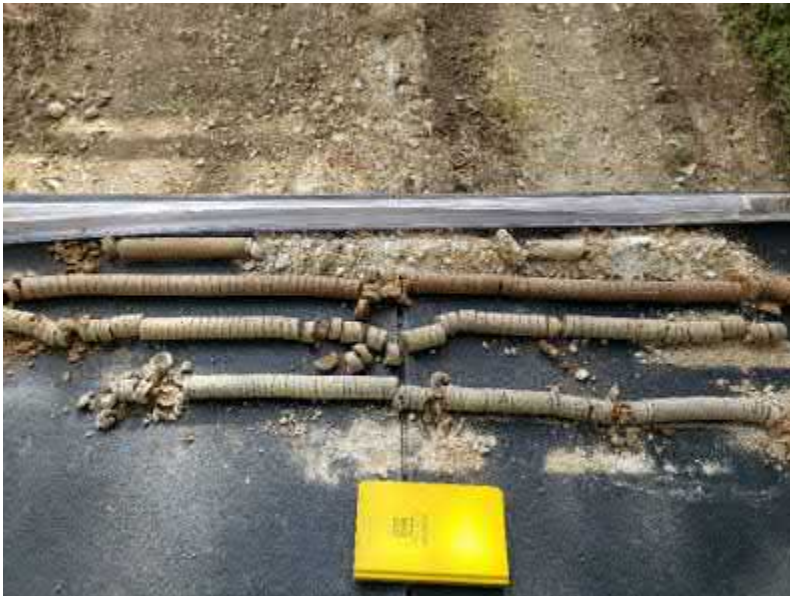
Photo #19 Typical view of soil cores collected from soil boring B-7.
