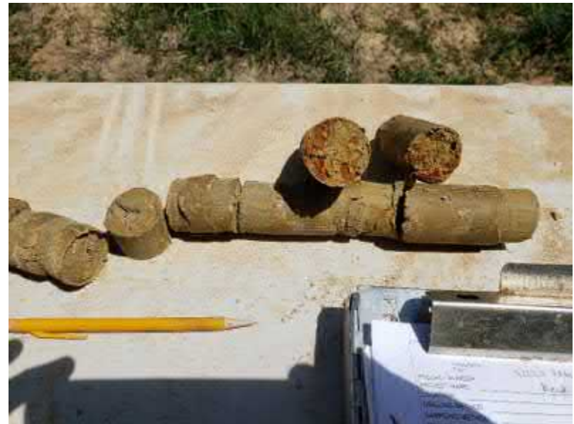
Photo #16 View of Navaro clay encountered at the bottom of the soil boring MM-6.
