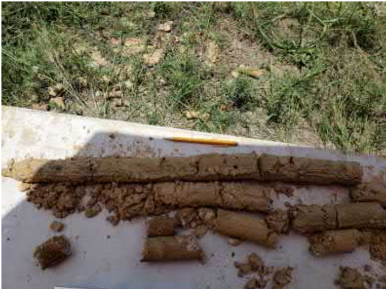
Photo #7 View of soil sample from the bottom of the soil boring MM-2, showing Navaro Clay present.
