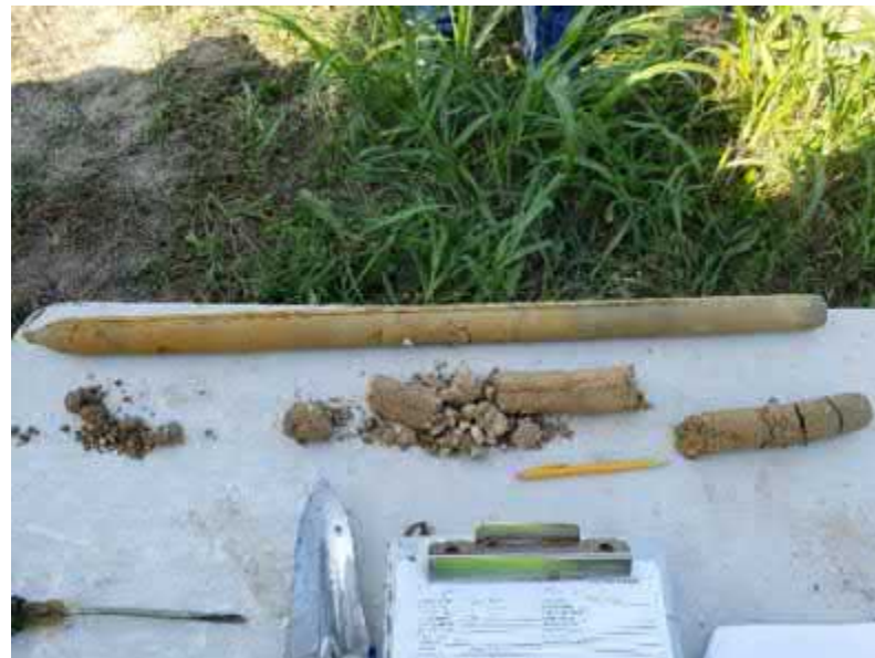
Photo #2 View of typical soil sample collected from the soil boring MM-1.
